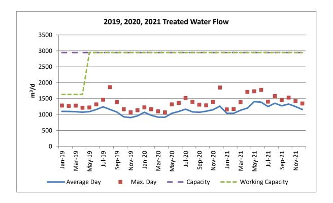
Maximum treated water demand was observed in June 2021. The cause is due to annual hydrant flushing and maintenance.. During 2021, there were three service leak repairs, one hydrant replacement and no watermain break repairs Repair or PM replacement of one customer service valve was also completed in 2021 along with two new service connections.
